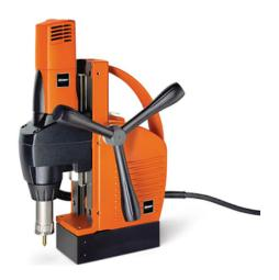
Holes from 7/16" (12 mm) to 1 1/4" (32 mm) diameter can be made with the JCM 125 Q. The JCM125Q is ideal for installation work on site due to its compact dimensions and low weight of only 23.1lbs (10.5kg).
