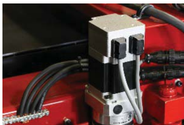
Planetary Gearbox and Servo Motor Precise and accurate motion
