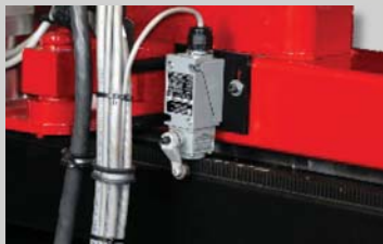
Limit Switches Used for machine over-travel as well as homing.
