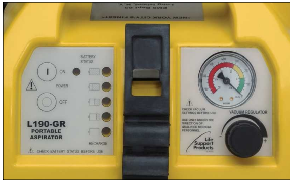
L190-GR LEDs indicate status of battery charge. Increase vacuum by turning regulating knob clockwise.
